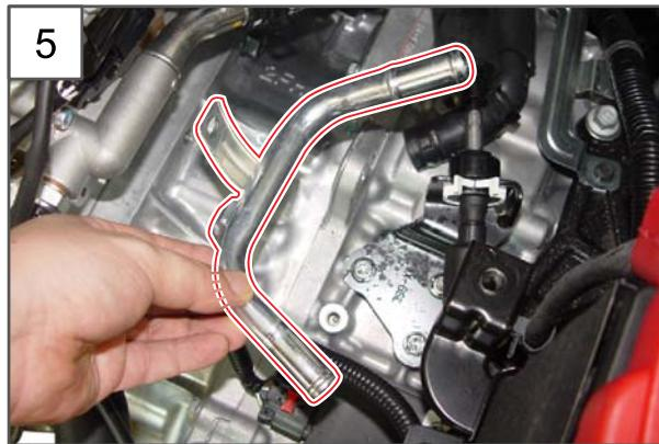
5. Remove the TOC coolant supply pipe.
