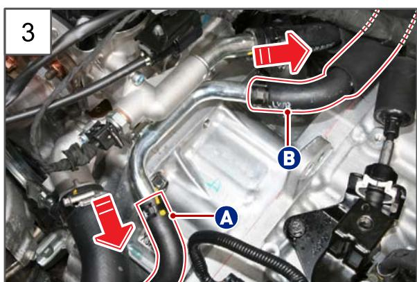
3. Disconnect the TOC coolant supply hose (A) and heater lower hose (B) from the TOC coolant supply pipe.
